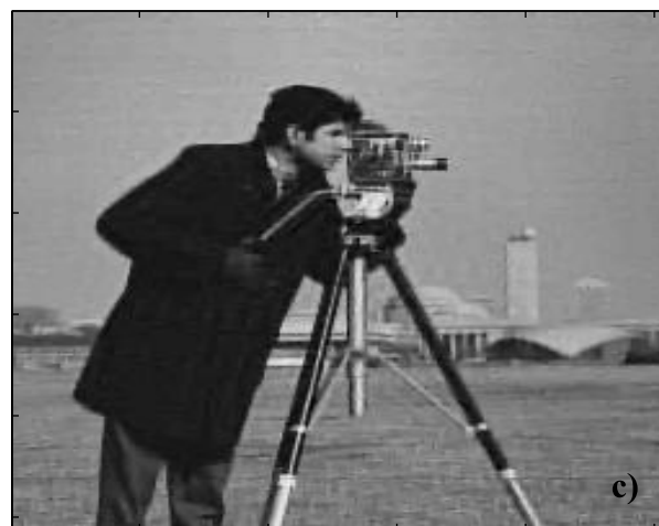
Fig. 2. Camera-man: a) Original image; b) Blurred noisy image (blur (9 \times 9) uniform, BSNR=40 dB); c) Restored image with Algorithm 1 (ISNR = 8.1dB).
