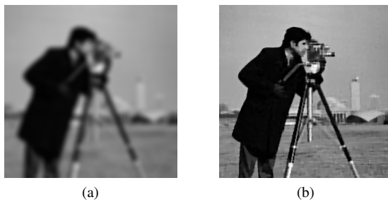
Fig. 5. Deblurring: observed (a) and estimated (b) images using the Proposed-AD method. The experiments were run for the cameraman image with a 13 \times 13 boxcar blur.
