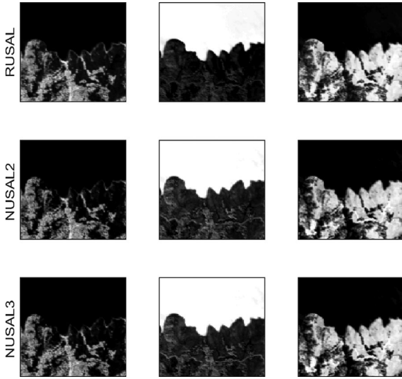
Fig. 4. Estimated abundance maps with different algorithms for the Moffett image. (Left) vegetation, (middle) water, (right) soil.
