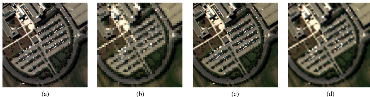
Fig. 9. Results for data set B (HSI + MSI fusion). All images are in false color. (c) and (d) are very similar to (a) due to the false color rendering, but they have 93 bands, whereas (a) has only four. (a) Observed MSI. (b) Observed HSI. (c) HySure's result. (d) ZBS's result.
