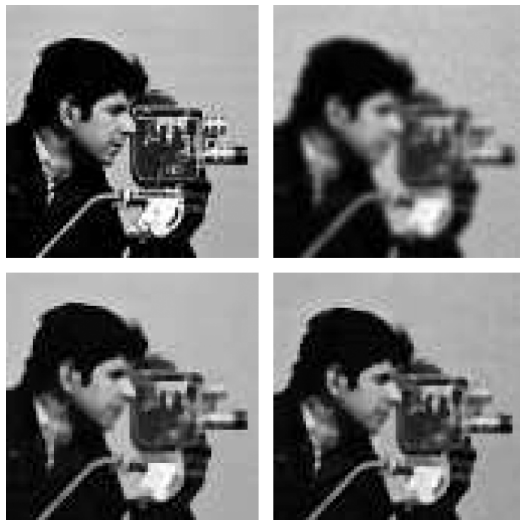
Fig. 7. Experiment of Section VI-A. Top row: (left) original; (right) blurred and noisy image. Bottom row: estimate from [50]; estimate by PIDAL-TV (ISNR = 4.8 dB).
