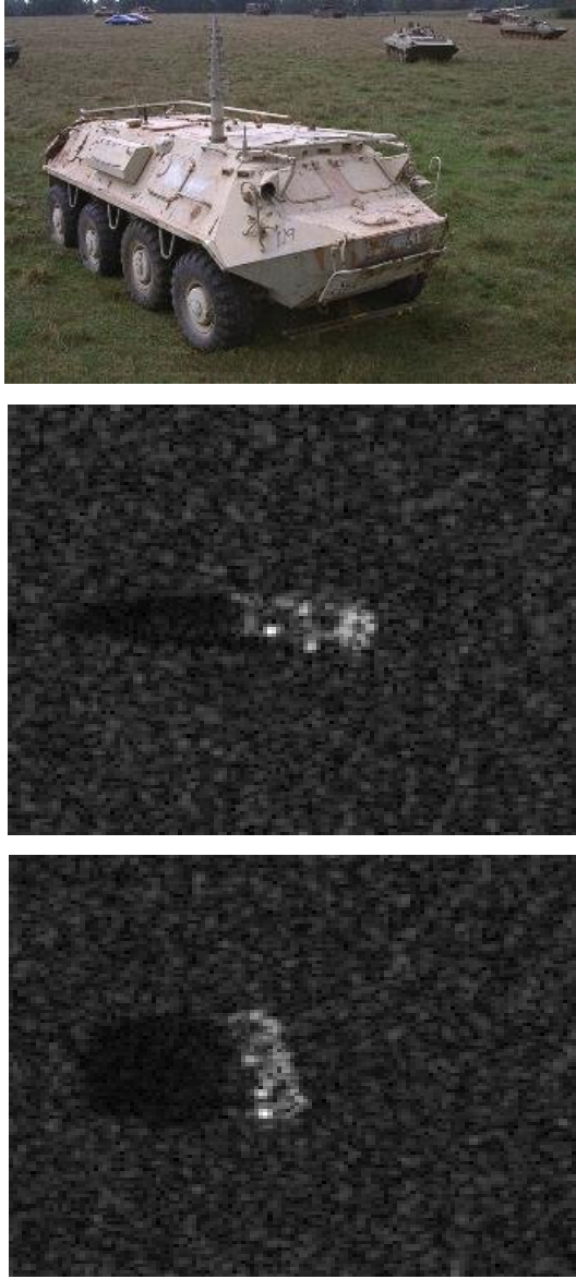
Fig. 10. Visible (top) and X-Band (middle and bottom) images of the BTR 60 transport vehicle (data from the MSTAR data public collection). Aspect angles of the middle and bottom images are nearly 0^\circ and 90^\circ , respectively.
